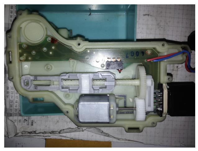
It's just about the motor at the bootom - a Mabuchi FC-280PD-20150. This motor is not thermistor protected. It showed very erratic DC resistances of several hundred Ohms. Once removed from the structure, I could however run it easily in both directions from 12 V DC.
