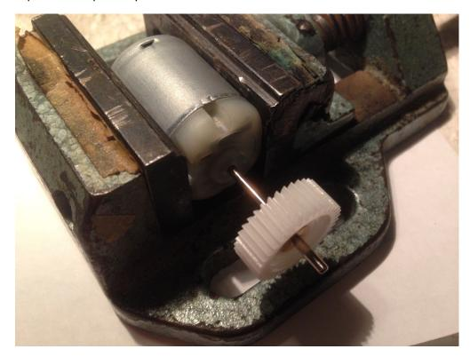
The reassembled motor had 0.6 k $\Omega$  DC resistance and took idle-running 0.11 A from 12 V DC.
